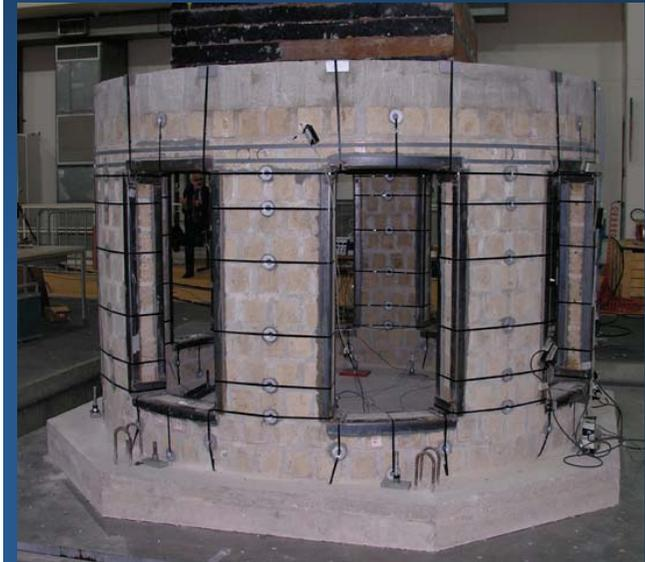
Dissipative frames couplet with CAM system
